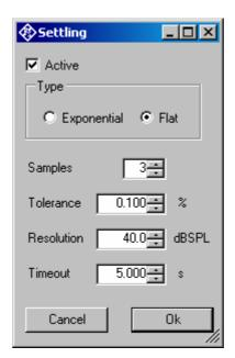
Fig. 11 Input window for adaptive measurement
