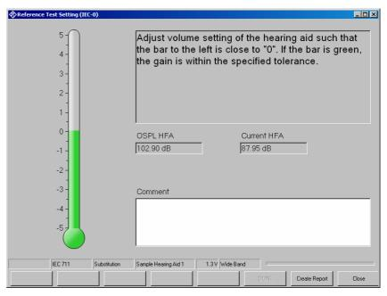
Fig. 47 Display of the routine for reference test gain setting, adjusted
