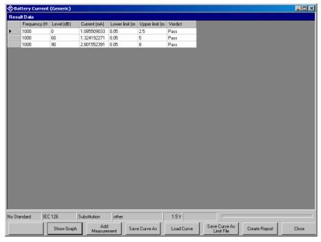
Fig. 43 Value table display of battery current measurement
