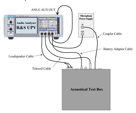
Fig. 1 Test setup and connection of external components
