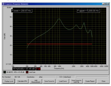
Fig. 31 Display window of frequency response measurement
