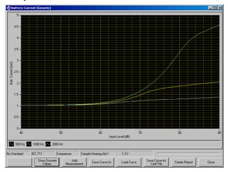
Fig. 42 Graphic display of battery current measurement
