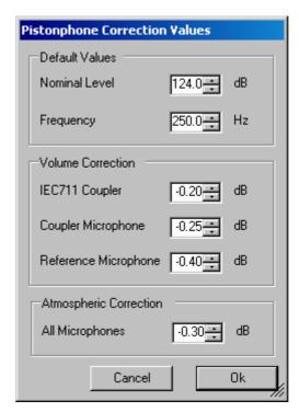
Fig. 19 Input window pistonphone correction values
