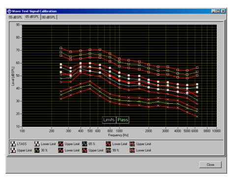
Fig. 21 ISTS calibration result
