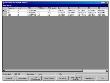
Fig. 37 Data table display of harmonic distortion measurement
