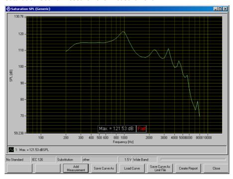
Fig. 35 Display window of saturation sound pressure level measurement
