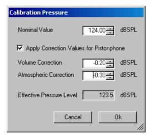
Fig. 17 Input window for calibration SPL
